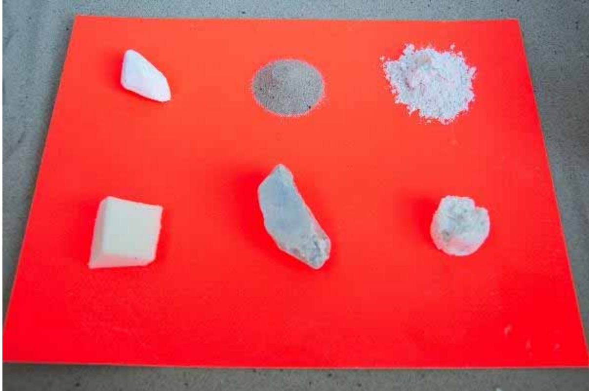
(fig. 32 Used materials: from top left: Magnesium, Sand, Plaster, PU-foam, Steatite, Magic-Sand)
