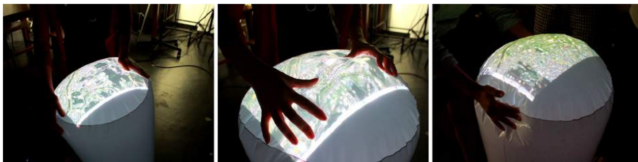
Fig. 16 Left navigating the map by tilting the prototype. Middle grabbing the actual screen to view the specific location precisely. Right grabbing the prototype on its side with two hands to zoom in the map
