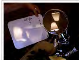
Real image of a lamp is projected onto a screen (inverted). Reflections of the lamp from both surfaces of the biconvex lens are visible.
