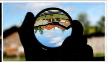
A convex lens ( f \ll S_1 ) forming a real, inverted image rather than the upright, virtual image as seen in a magnifying glass
