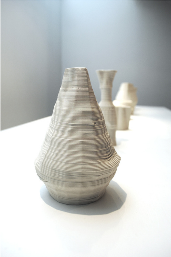
L'Artisan Electronique, Unfold / Tim Knapen / RepRap Community 3D printed vase with flaws
